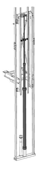
For travel heights of up to 11 meters ALGI are pleased to announce the new TAZ system. The heart of this innovative design is the free-floating cylinder support. ALGI have been able to engineer a cost effective solution whilst also improving performance and safety. Our proven telescopic cylinder designs with all of its comfort and safety benefits will be more than competitive with other hydraulic and traction systems.
